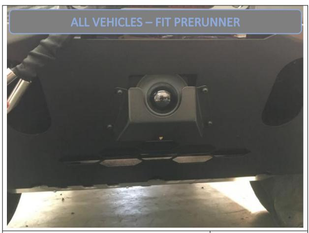
64. Secure ACC cover to main plate with M6x16 button head cap screws washers and flange nuts.
