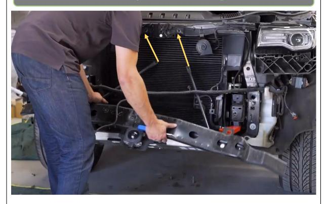
26. Remove 2x screws with 13mm tool holding round support bars from top of bonnet support then remove entire reinforcement bar.
