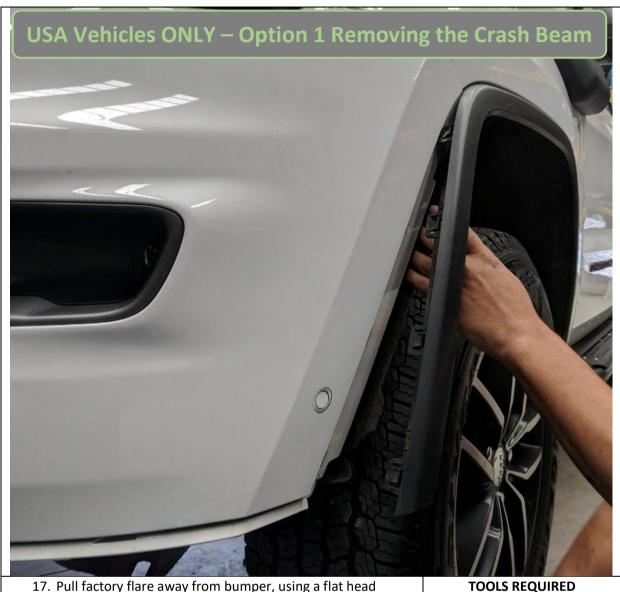
17. Pull factory flare away from bumper, using a flat head screwdriver release at least 2 of the push in clips on top edge being careful not to break them as you pull the flare away from the body.
