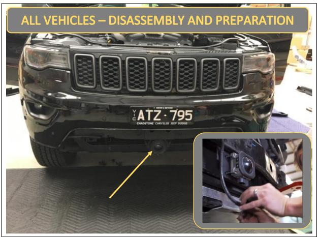
9. If Adaptive cruise control is fitted, unplug loom and pull sensor off the mounting posts.
