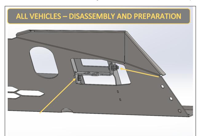
12. Fit the Pre runner mount brackets to Tow Points as shown with M10x25 bolts, washers and flange nuts.
