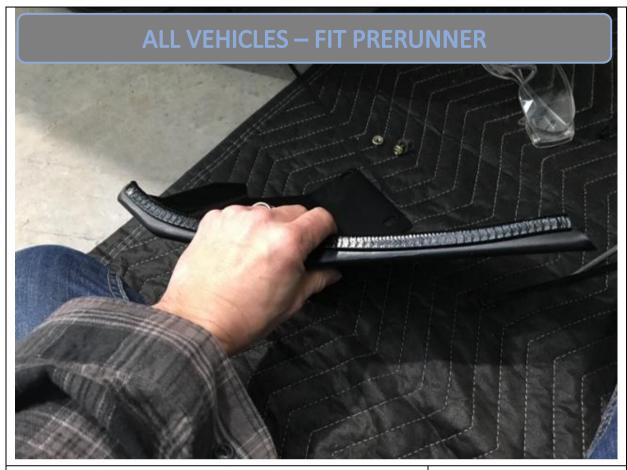
52. Fit pinch weld to top edge of wings like shown
