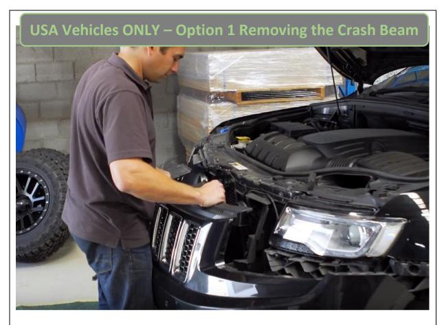
20. Lifting the top section ever so slightly you can release clips holding in the top section and pull the remainder of the bumper away.
