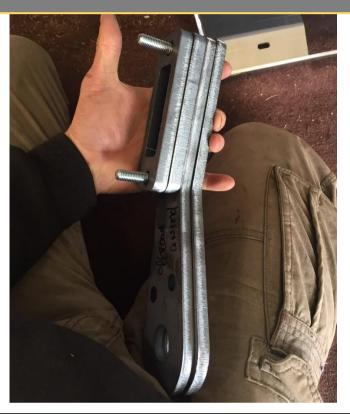
6. Stack Offroad Animal Tow points together as shown with M10 bolts and M10 flat washers.
