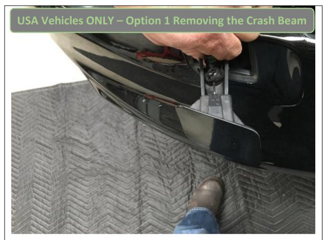
18. Pull headlight washer out by hand and detach retaining clips allowing mechanism to retract and remove outside panel.
