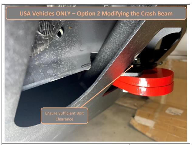
42. Re-fit the tow points then fit Prerunner center plate. There should be sufficient clearance such that the Prerunner does not touch the crash beam, and that the M10x45 bolts can pass easily through the mount and tow point.
