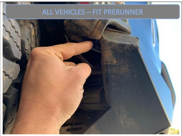
69. If your Jeep is equipped with parking sensors and they are going off as they see the new bumper you can fix this by adding a cable tie to the slot that originally holds the lower air dam being pointed to in the picture.
