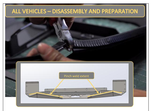
11. Prepare the Prerunner plate for fitment. First Fit Pinch weld to top edges of Prerunner plate. Trim edges of pinch weld at edge of plate.
